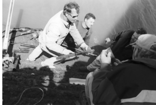
Crew pulling foundation core samples
